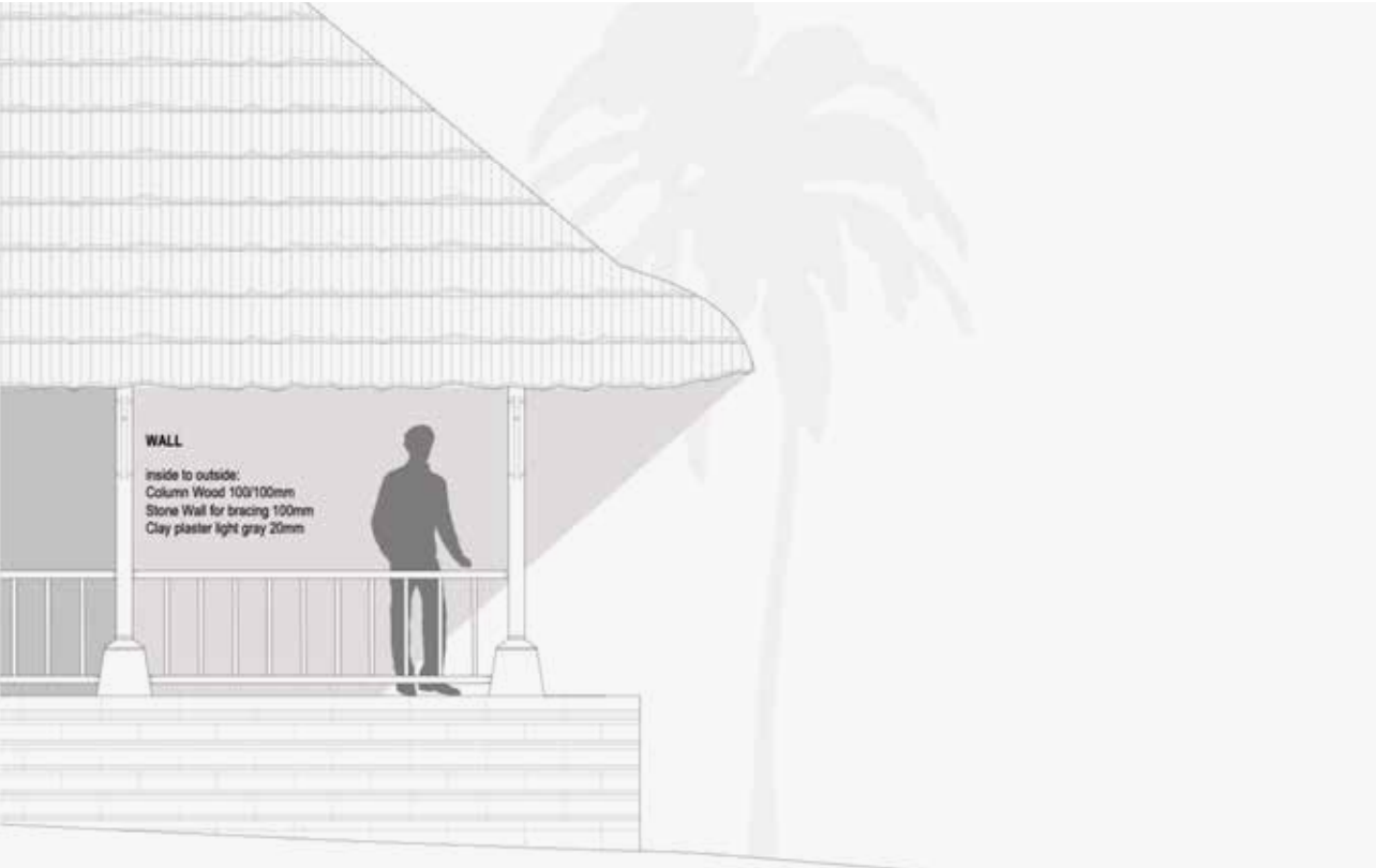
Part elevation I construction 1:20
