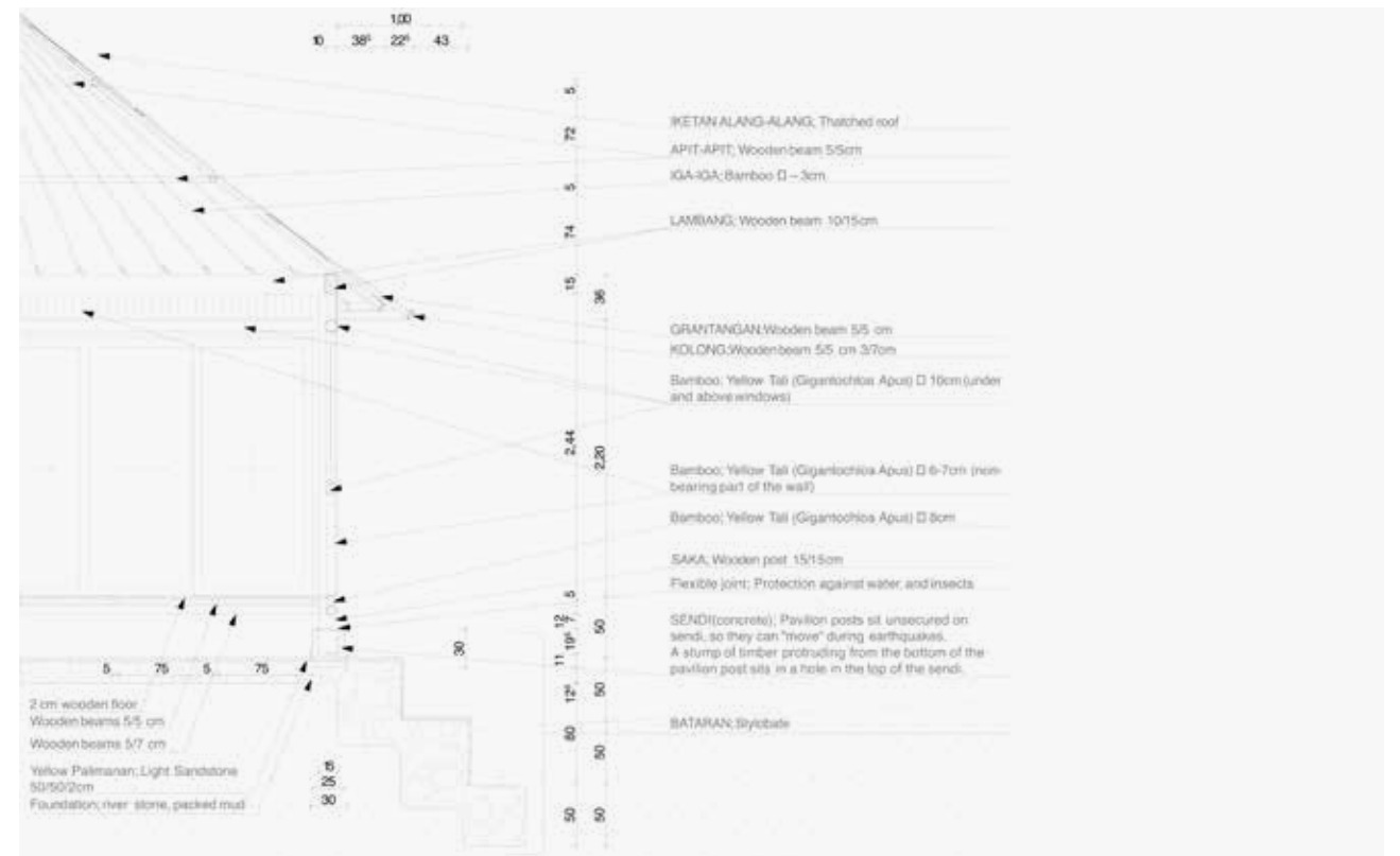
Facade section I construction 1:25
